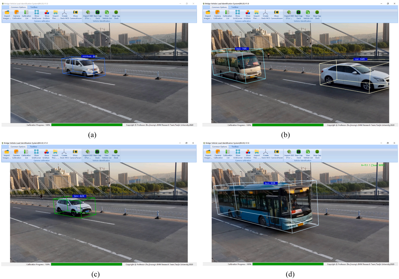
Fig. 11. Reconstruction of vehicle 3D bounding box: (a) Wuling Hongguang (minibus); (b) Chevrolet Cruze (car); (c) Mitsubishi Outlander (SUV); (d) Urban bus (bus).
